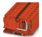
Feed-through terminal block, nom. voltage: 1000 V, nominal current: 125 A, number of connections: 2, connection method: Spring-cage connection, Rated cross section: 35 mm $^2$ , 1 level, cross section: 2.5 mm $^2$  - 35 mm $^2$ , mounting type: NS 35/7,5, NS 35/15, color: red
