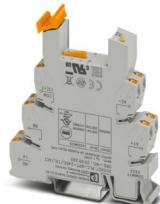
14 mm PLC basic terminal block for high switch-on currents with push-in connection, without relay or solid-state relay, for mounting on DIN rail NS 35/7,5, with load return line connection (BB), 1 N/O contact, input voltage 24 V DC
