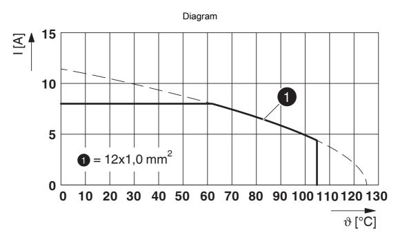
I = current strength,  $\vartheta$  = ambient temperature, 12x 8 A
