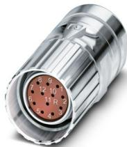
M23, Cable connector, series: CA, straight, shielded: yes, Screw locking mechanism, No. of pos.: 12, Direction of rotation: Counter direction, contact connection type: Socket, Crimp connection, cable diameter range: 4 mm ... 6 mm, coding: N. This product is in the process of being discontinued. This product must no longer be considered for new projects. Please contact your sales representative for alternatives.
