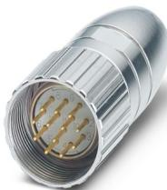
M23, Cable connector, straight, Screw locking mechanism, No. of pos.: 17, Direction of rotation: Standard, contact connection type: Pin, Solder cup, cable diameter range: 7.5 mm ... 9.5 mm, coding: N
