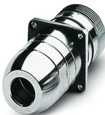
M23, Rear panel feed-through, series: RC, straight, shielded: yes, Screw locking mechanism, No. of pos.: 12, Direction of rotation: Standard, contact connection type: Pin, Solder cup, Radial O-ring, Panel thickness max.: 2.5 mm, cable diameter range: 6.5 mm ... 7.5 mm, coding: N. This product is in the process of being discontinued. This product must no longer be considered for new projects. Please contact your sales representative for alternatives.
