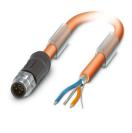
Bus system cable, FOUNDATION Fieldbus (31.25 kbps), 3-position, PVC, orange RAL 2003, shielded, Plug straight M12, coding: A, on free cable end, cable length: 15 m
