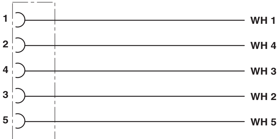
Contact assignment of the M12 socket
