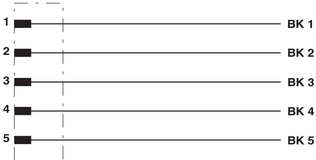
Contact assignment of the M12 socket
