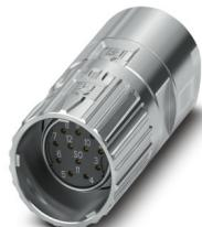
M23, Cable connector, series: M23 PRO, straight, shielded: yes, ONECLICK fast locking system, No. of pos.: 12, Direction of rotation: Counter direction, contact connection type: Socket, Crimp connection, cable diameter range: 6 mm ... 10 mm, coding: N, Item is lead-free in accordance with RoHS II without Exemption 6c (Pb < 0.1 %)
