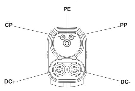
Pin assignment of the Vehicle Connector
