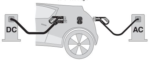
The Combined Charging System (CCS) principle - standard-compliant charging system for electric vehicles, which supports both conventional AC charging and fast DC charging. Both Vehicle Connectors fit into the CCS Vehicle Inlet.
