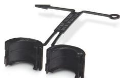
Locking clip for the male and female side of sensor/actuator cables with straight M12 connector and M12 connectors designed for assembly featuring QUICKON fast connection technology, used to secure M12 connectors in areas with a danger of dust explosions in zone 22 in accordance with EN 50281-1-1
