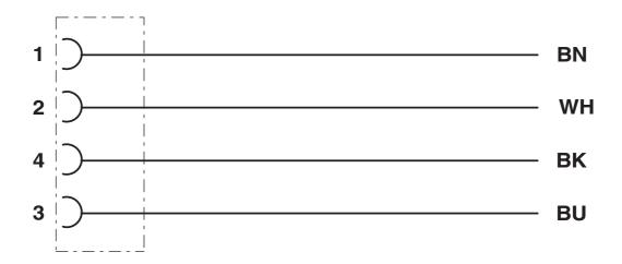
Contact assignment of M8 socket
