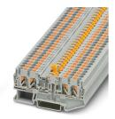
Knife-disconnect terminal block, nom. voltage: 400 V, nominal current: 20 A, 1 level, connection method: Push-in connection, Rated cross section: 2.5  $\text{mm}^2$ , cross section: 0.14  $\text{mm}^2$  - 4  $\text{mm}^2$ , mounting: NS 35/7,5, NS 35/15, color: gray
