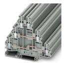
Multi-level terminal block, nom. voltage: 500 V, nominal current: 19 A, connection method: Screw connection, Rated cross section:  $2.5 \text{ mm}^2$ , cross section:  $0.14 \text{ mm}^2$  -  $4 \text{ mm}^2$ , mounting type: NS 35/7.5, NS 35/15, color: gray
