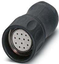
M23, Cable connector, series: RC, straight plastic-sheathed, shielded: yes, Screw locking mechanism, No. of pos.: 17, Direction of rotation: Standard, contact connection type: Socket, Crimp connection, cable diameter range: 6.5 mm ... 7.5 mm, coding: N
