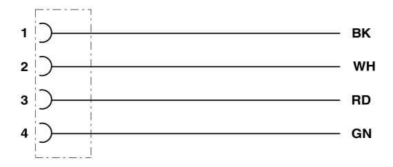
Contact assignment of 7/8" socket
