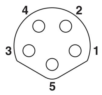
Pin assignment of M8 socket, 5-pos., B-coded
