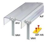
Flat-ribbon cover, for covering terminal strips, 2 mm thick, 17,5 cm wide, an additional requirement are 2 E/UK end brackets and 2 adjustable VAH cover holders. The max. supply length is 100 cm
