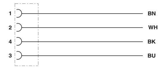
Contact assignment of M8 plugs/sockets
