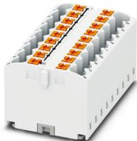
Distribution block, Basic terminal block, nom. voltage: 450 V, nominal current: 24 A, number of connections: 18, connection method: Push-in connection, cross section: 0.14 mm<sup>2</sup> - 4 mm<sup>2</sup>, mounting type: for snapping onto a DIN rail adapter, Direct mounting with flange, Free-hanging, color: white
