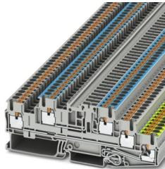
Installation protective conductor terminal block, nom. voltage: 400 V, Thermal continuous current  $I_{th}$ : 22 A, Push-in connection, Rated cross section: 2.5 mm<sup>2</sup>, cross section: 0.14 mm<sup>2</sup> - 4 mm<sup>2</sup>, Push-in connection, Rated cross section: 2.5 mm<sup>2</sup>, cross section: 0.14 mm<sup>2</sup> - 4 mm<sup>2</sup>, mounting type: NS 35/7,5, NS 35/15, color: gray
