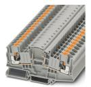
Component terminal block, for installing components that can be individually selected, nom. voltage: 500 V, nominal current: 30 A, connection method: Push-in connection, 1 level, Rated cross section:  $6~\text{mm}^2$ , cross section:  $0.5~\text{mm}^2$  -  $10~\text{mm}^2$ , color: gray
