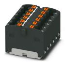
Distribution block, bridged internally, nom. voltage: 450 V, nominal current: 17.5 A, number of connections: 12, connection method: Push-in connection, cross section: 0.14 mm<sup>2</sup> - 2.5 mm<sup>2</sup>, mounting type: for snapping onto a DIN rail adapter, Direct mounting with flange, Free-hanging, color: black
