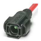
Device connector front mounting, Range of articles: SUNCLIX, housing material: PPE, color: black, min. conductor cross-section: 4 mm², rated current: 40 A, Connection method: Crimp, cable length: 100
