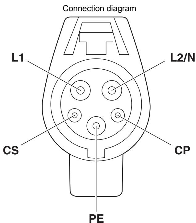
Pin assignment of the Vehicle Connector
