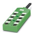
Distributor box, application: Standard, extended requirements, connection method: M12 socket Metal, number of slots: 8, number of positions: 4, coding: A, slot assignment: single, status display: no, Universal; master cable connection: Fixed connection 180°, PUR/PVC, cable length: 5 m, shielding: no
