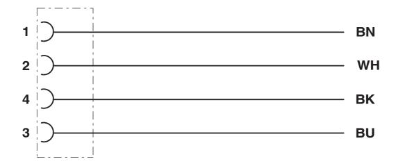
Contact assignment of M8 socket
