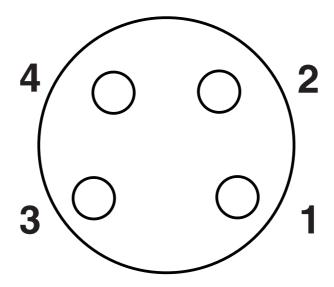
Pin assignment M8 socket, 4-pos.
