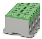
High-current terminal block, nom. voltage: 1000 V, nominal current: 380 A, number of connections: 2, number of positions: 1, connection method: Screw connection, Rated cross section: 240 mm<sup>2</sup>, cross section: 35 mm<sup>2</sup> - 240 mm<sup>2</sup>, Rated cross section: 240 mm<sup>2</sup>, cross section: 35 mm<sup>2</sup> - 240 mm<sup>2</sup>, mounting type: Screw mounting, color: green
