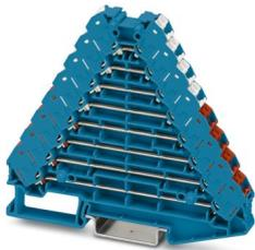
Potential distributors, without actuating push button, nom. voltage: 250 V, nominal current: 17.5 A, connection method: Push-in connection, 1st, 2nd, 3rd and 4th level, Rated cross section: 1.5 mm<sup>2</sup>, cross section: 0.14 mm<sup>2</sup> - 2.5 mm<sup>2</sup>, mounting: NS 35/7,5, NS 35/15, color: blue, color of connection elements: white, red
