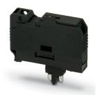
Fuse plug, Prior to replacing the cartridge fuse, disconnect the fuse connector from the basic terminal block., nom. voltage: 500 V, nominal current: 10 A, connection method: Plug-in connection, fuse type:  $G/6.3 \times 32$ , color: black
