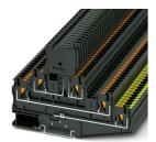
Fuse modular terminal block, fuse type: Glass / ceramics / ..., fuse type: G / 5 x 20, nom. voltage: 24 V, nominal current: 6.3 A, connection method: Push-in connection, Rated cross section: 4 mm $^2$ , cross section: 0.2 mm $^2$ - 6 mm $^2$ , connection method: Push-in connection, cross section: 0. 2 mm $^2$ - 6 mm $^2$ , mounting type: NS 35/7,5, NS 35/15, color: black
