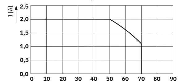
Maximum permissible current per path in uncoiled state
