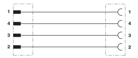
Contact assignment of M8 plugs/sockets
