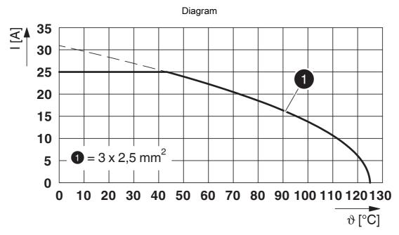
I = current strength, ϑ = ambient temperature, 3x 25 A
