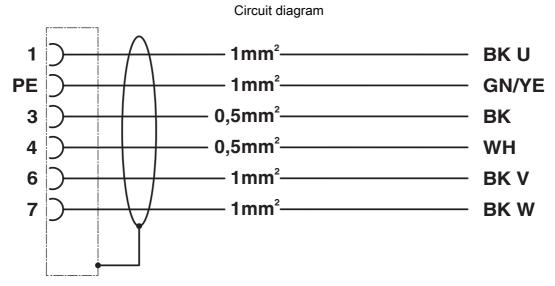
Contact assignment of M17 plugs/sockets, cable type C01
