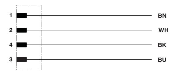
Contact assignment of the M12 plug
