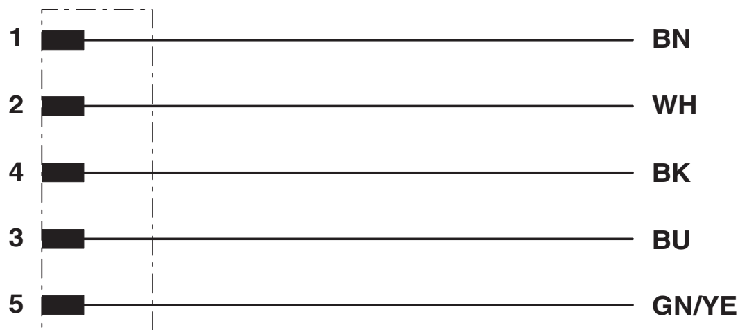
Contact assignment of the M12 plug
