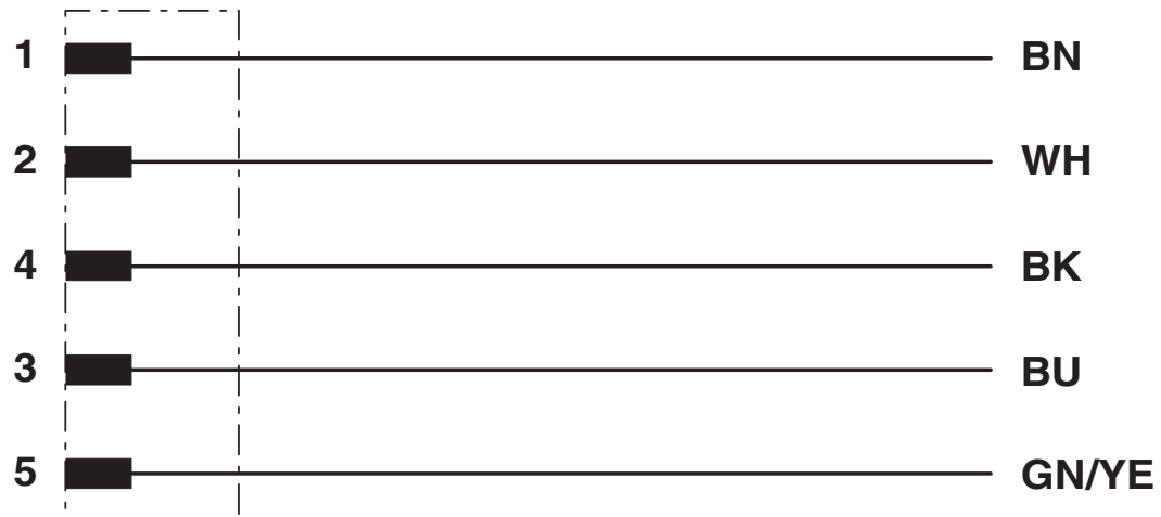
Contact assignment of the M12 plug
