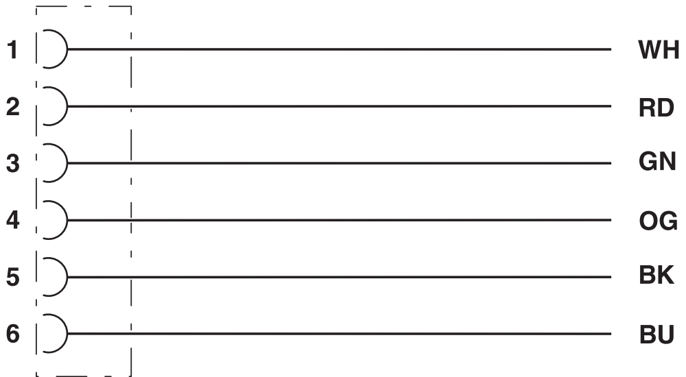
Contact assignment of 7/8" socket
