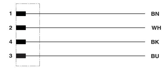
Contact assignment of the M12 plug
