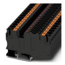
Fuse modular terminal block, fuse type: Blade, fuse type: C, nom. voltage: 24 V, nominal current: 25 A, connection method: Push-in connection, Rated cross section: 10 mm<sup>2</sup>, cross section: 0.5 mm<sup>2</sup>- 16 mm<sup>2</sup>, mounting type: NS 35/7,5, NS 35/15, color: black
