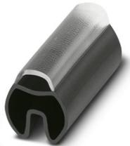
Conductor marker carrier, transparent/black, unlabeled, cable diameter range: 4 ... 7 mm, mounting type: slide-on, text field height: 4 mm, text field width: 18 mm
