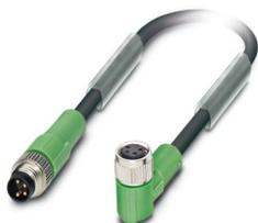
Sensor/actuator cable, 4-position, PUR halogen-free, black-gray RAL 7021, Plug straight M8, coding: A, on Socket angled M8, coding: A, cable length: 3 m
