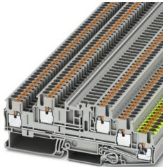
Installation protective conductor terminal block, Current and voltage are determined by the plug used., nom. voltage: 400 V, nominal current: 22 A, Push-in connection, Rated cross section: 2.5 mm<sup>2</sup>, cross section: 0.14 mm<sup>2</sup> - 4 mm<sup>2</sup>, Push-in connection, Rated cross section: 2.5 mm<sup>2</sup>, cross section: 0.14 mm<sup>2</sup> - 4 mm<sup>2</sup>, mounting type: NS 35/7,5, NS 35/15, color: gray
