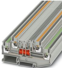
Disconnect terminal block, Current and voltage are determined by the plug used., with isolating plug, nom. voltage: 400 V, nominal current: 16 A, 1st and 2nd level, connection method: Push-in connection, Rated cross section: 2.5 mm<sup>2</sup>, cross section: 0.14 mm<sup>2</sup> - 4 mm<sup>2</sup>, mounting: NS 35/7,5, NS 35/15, color: gray
