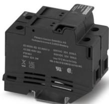
Fuse holder, fuse type: Ceramic, fuse type: 10.3 x 38 mm, nom. voltage: 690 V AC, nominal current: 32 A, number of positions: 2, connection method: Screw connection, Rated cross section: 16 mm<sup>2</sup>, cross section: 1 mm<sup>2</sup> - 16 mm<sup>2</sup>, mounting type: NS 35/7,5, NS 35/15, color: black
