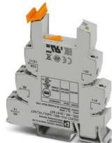
14 mm PLC basic terminal block for high switch-on currents with screw connection, without relay or solid-state relay, for mounting on DIN rail NS 35/7,5, with load return line connection (BB), 1 N/O contact, input voltage 24 V DC
