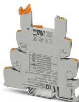
6.2 mm PLC basic terminal block with Push-in connection, without relay or solid-state relay, for mounting on DIN rail NS 35/7,5, 1 changeover contact, input voltage 24 V DC
