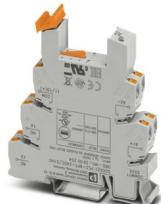
14 mm PLC basic terminal block for high continuous currents with Push-in connection, without relay or solid-state relay, for mounting on DIN rail NS 35/7,5, 1 changeover contact, input voltage 24 V DC
